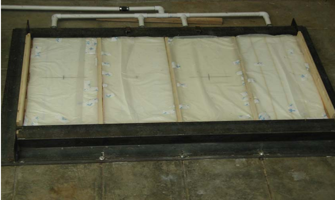
Figure 2. Pressure test apparatus without specimen installed (showing airbags).
