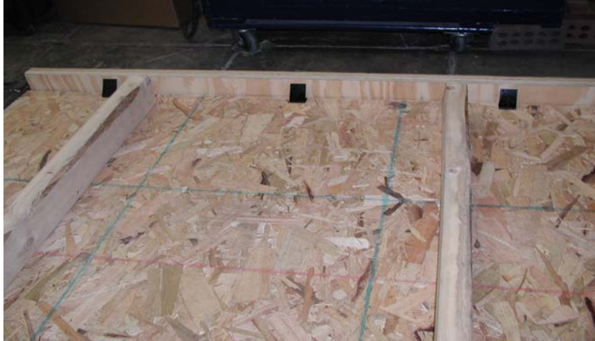
Figure 7. Pressure test of Plylox™ clips with 8 ft panel span and 2-2x4 stiffeners.
