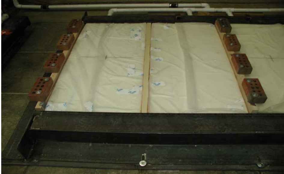
Figure 5. Pressure test set-up with sand-faced clay brick opening recess material (nominal 4 foot panel with Plylox™ clips not shown).
