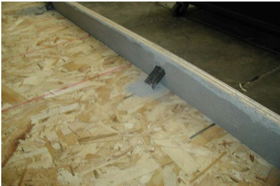
Figure 6. Pressure test of Plylox™ clips with Portland cement stucco opening recess finish material.
